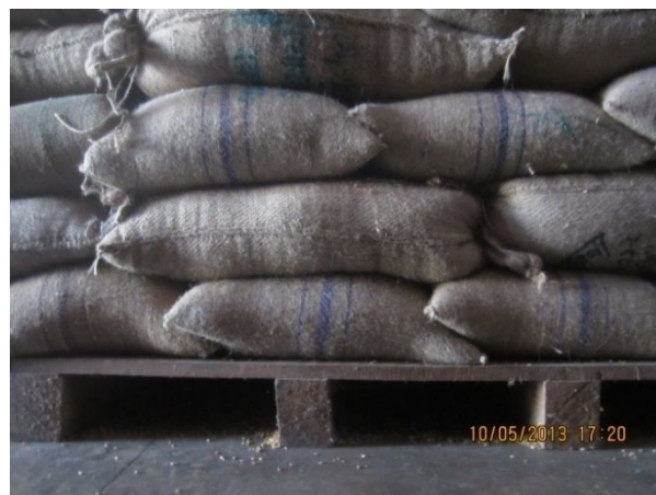
Plate 3.13: Use of wooden Dunnage for storage of food products in the godown of Sirajganj
